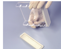
Rotate the Casting Tray and repeat the process with the other Silicone Casting Gate.
