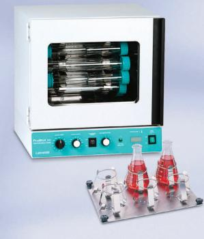
Specifications\*Catalog numberH-1200-SABottle capacity12 large, 24 smallExterior dimensions (WxDxH)19x17.5x19.5 in.Chamber dimensions (WxDxH)14.5x11x13.3 in.Temperature rangeAmbient +5° to 80°C\*See back page for information on bottles, platforms and other accessories
